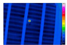
Thermal anomaly of bat roosting between tiles Bat flying over water with reflection and underfelt
